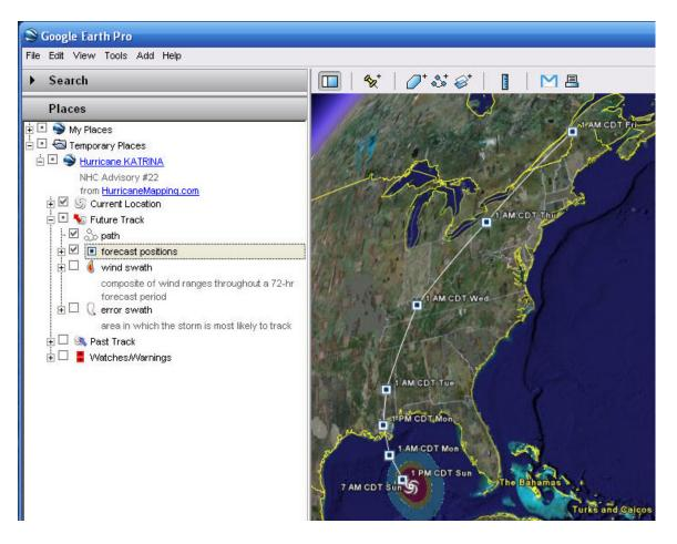
Shown below, we have expanded *forecast positions* item in the legend and double-clicked on the 36-hour forecast position. Google Earth flies into a closer view of that location and displays an information bubble containing storm statistics projected at that time.
